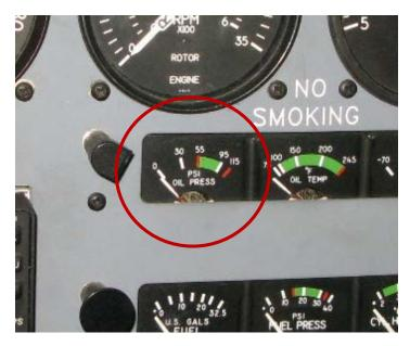
3. Check oil pressure to ensure proper operating pressure
