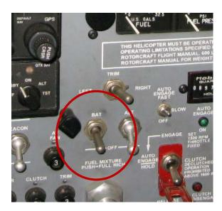
2. Switch battery switch (BAT) to the "On" position
